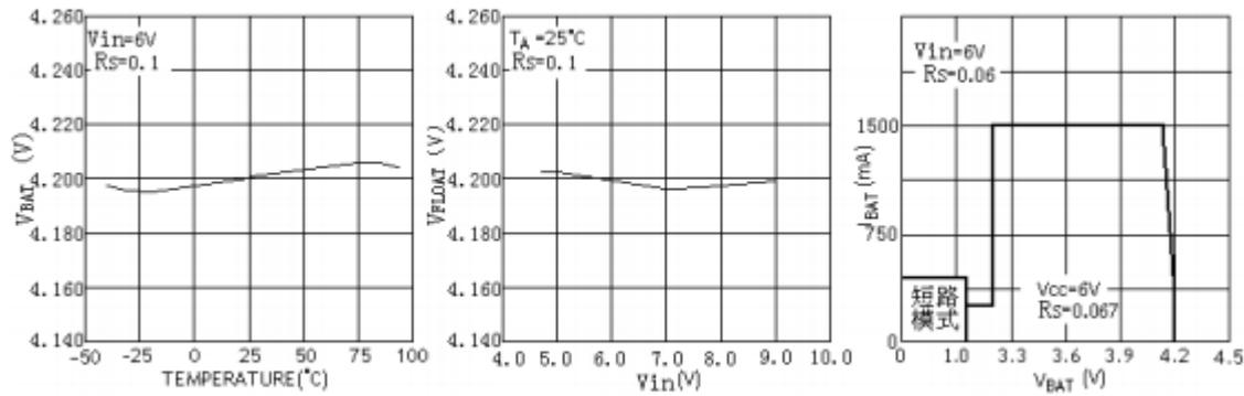
Cut-off voltage vs ambient temperature
