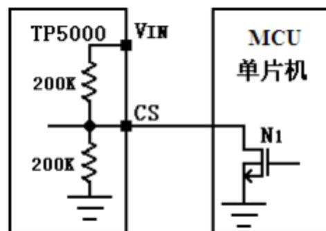
Figure 5 lithium iron phosphate battery charge status by external control Switching and stopping state
