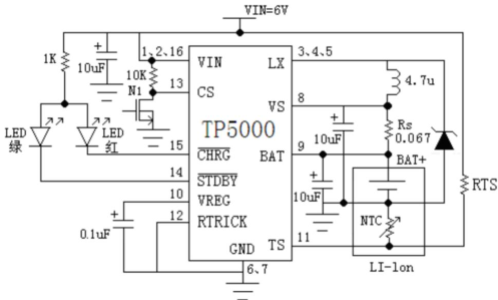
Figure 1 TP5000 is 1.5A 4.2V rechargeable lithium-ion battery (150MA prefill) Application Diagram
