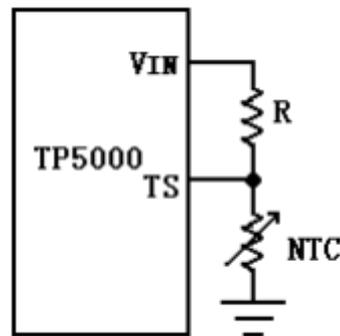
Figure 8 NTC connection diagram
