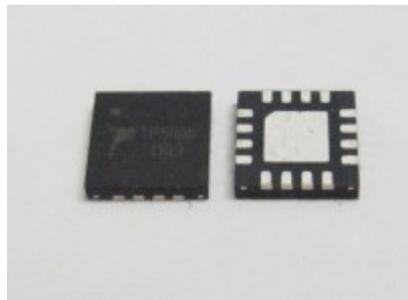
16-pin 4mm \* 4mmQFN16 Package Top View (Heat sink grounding unacceptable other potential)
